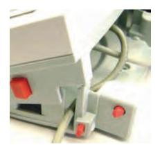
Thread printer cable along cable coils on bottom of balance. Or pass cable through groove near release button.
