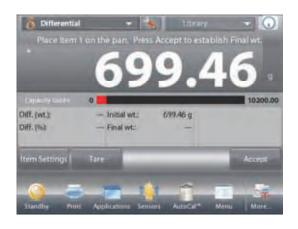
After **Accept** is pressed, the difference between initial and final weights appears in the Reference Fields.
