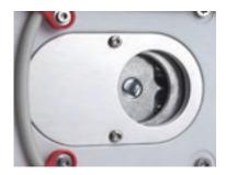
The balance can be supported using lab jacks or any other convenient method. Ensure the balance is level and secure. Power on the Balance, then use a string or wire to attach items to be weighed.
