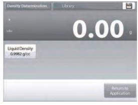
Measure the actual liquid density of the Density setup and enter it.
