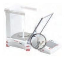
Press button to separate Terminal from Base. Seat panel's hooked ends in base. Swing panel to vertical position.
