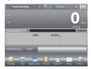
Press the Setup (wrench) button to enter the Counting Setup menu.
