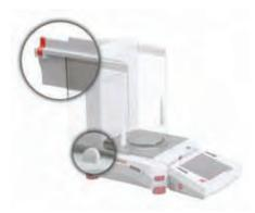
Position glass door to slide. Open lock tab (top); insert in top groove and slide inside bottom groove. Close lock tab.
