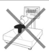
Do not allow any liquids to come into contact with the scale.
