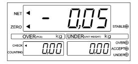
The tare weight can also be subtracted by pressing the TARE key after placing a tare weight on the weighing platter. Tare weight subtraction is also available by calling a preset weight. (Operation: Ref., 6-2 Calling a Preset Value)
