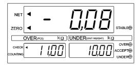
The upper and lower limit weights can also be set by calling preset values. To change a preset value temporarily, key in a new value and then press the over key or key.
