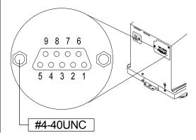
Singal names of the balance side are the same as the DTE side with TXD and RXD reversed.
