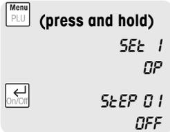
1. Press and hold the **Menu** (PLU) key until a long beep can be heard. SET 1 OP is displayed for "Operator Setup"
