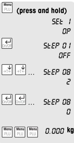
**Example: Setting digital filter to low (operator setup Step 8 = 0)**
