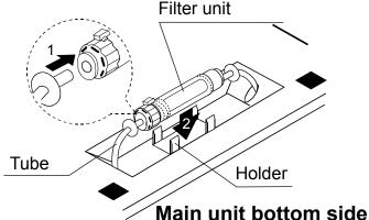
\* If particles of dust invade the tube, they may cause trouble. When replacing the filter, be careful that no dust invades the instrument.
