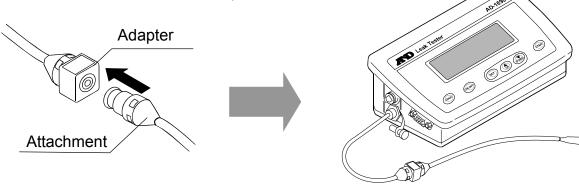
When the pipette does not match up with the attachment provided, replace the tip of the attachment with a tip that matches the pipette.
