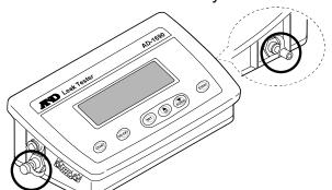
Confirm that the filter unit is installed in the holder located on the main unit bottom side correctly.
